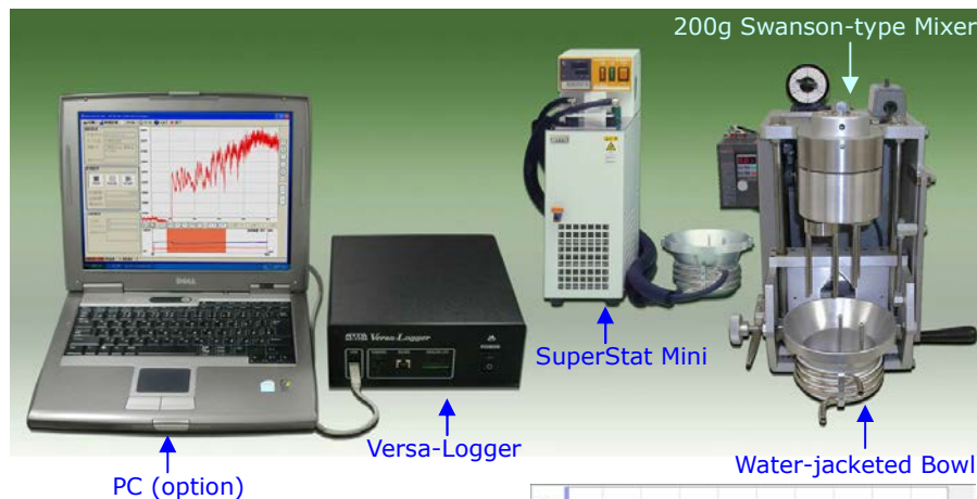
Fig.1. Versa-Logger System (center) with 200g Swanson-type Mixer (right)
